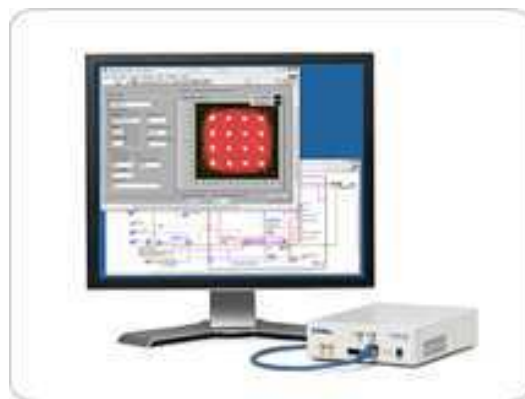
Figura 31. Universal Software Radio Peripheral (USRP) (Blossom., 2011)
