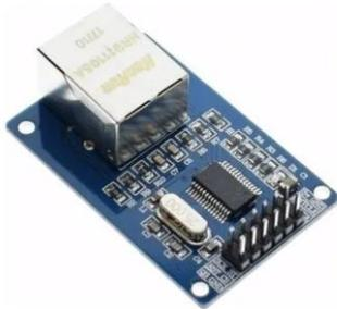
**Figura 8.** Modulo Ethernet Arduino (ELECTRONICSPOT, 2016)
