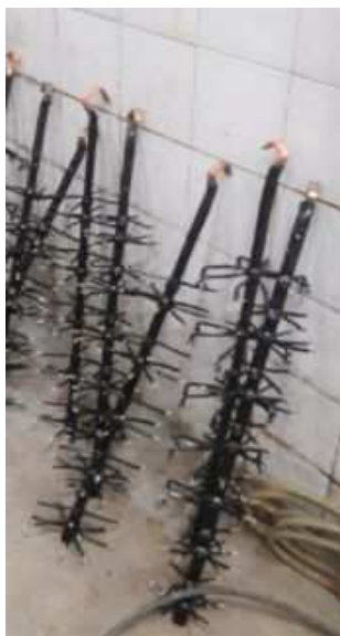
Figura 58. Gancheras previas a poka yoke.
