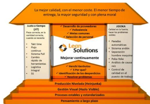
**Figura 9.** Casa Lean Manufacturing. Adaptado de Lean Solution (2019).
