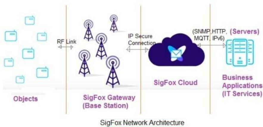
Figura 16. SigFox Network Architecture. Rfwireless-world (2020).
