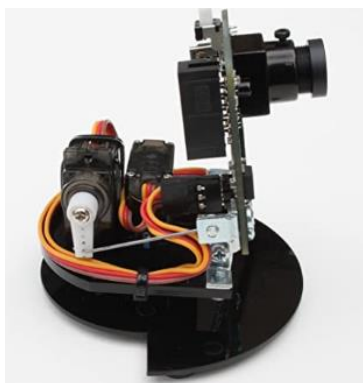
Figura 13. Pan/Tilt Servo Motor Kit (Amazon, 2020).
