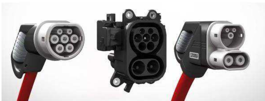
Figura 43. Conector combo 2. Wallbox (2019)
